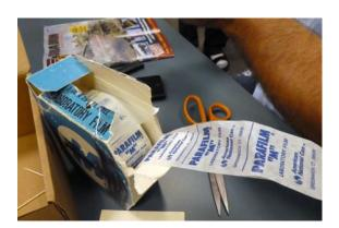
Parafilm is a polyurethane material with a wax layer on one side. Stretching the material creatures static electricity, which along with slight tackiness of the wax causes the film to stick to whatever it's applied to. Parafilm has been commonly used to mask canopies, and Rich demonstrated the technique.
