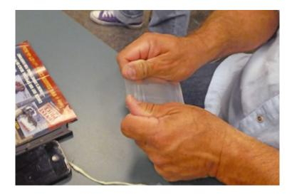
First, a section of material is cut a bit larger than the part to be masked. Then the film is stretched to activate the adhesive properties.
